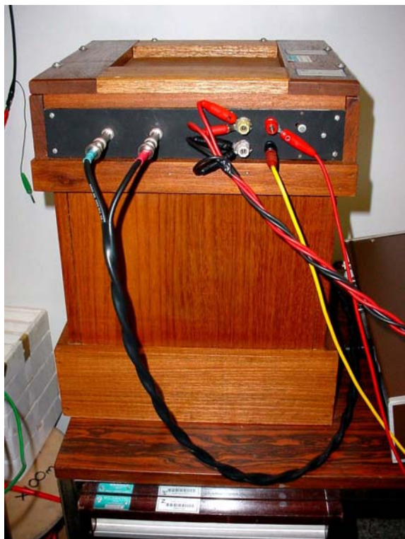
Fig. 3. Thermally-controlled standard capacitor.
