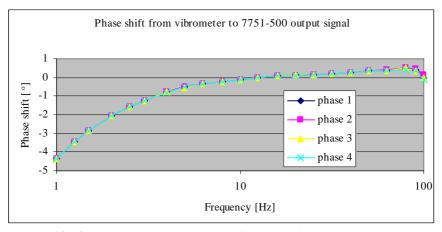
Fig. 10: Phase shift of the Endevco 7751-500 and vibrometer signals at each measurement point.
