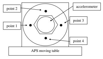
Fig. 7: Location of the measurement points.
