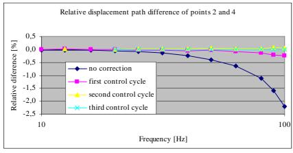
Fig. 11: Relative displacement between points 2 and 4.
