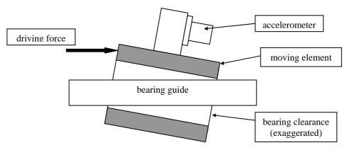
Fig. 5: Effect of the bearing clearance over the accelerometer.
