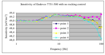
Fig. 9: Sensitivity of the Endevco 7751-500 calculated at each measurement point.
