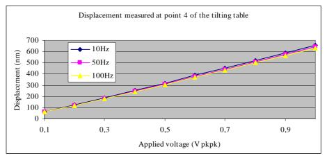
Fig. 8: Calibration of tilting table rotation versus applied voltage.
