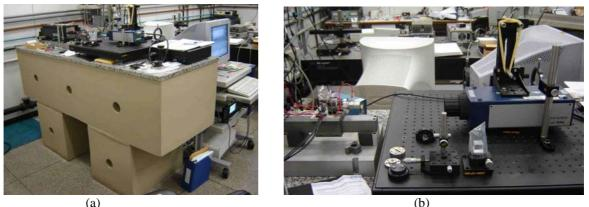
Fig. 4: View of the low frequency calibration system (a) and the APS-500 exciter (b).
