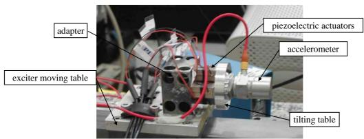
Fig. 3: View of the system mounted over the APS exciter.
