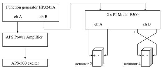
Fig 6: Electrical connections of the piezoelectric actuators.
