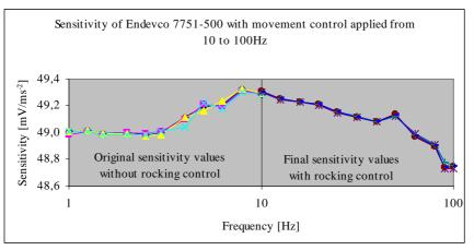
Fig 13: Final values of the sensitivity of accelerometer Endevco 7751-500.
