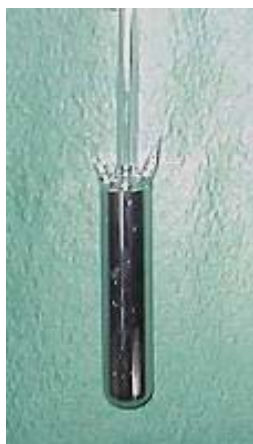
FIGURE 3 – Mercury triple point cell manufactured by Inmetro and Visomes (INM_VIS_03).
