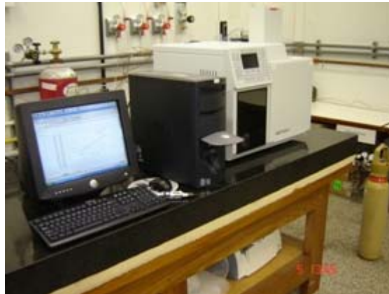
Figura 6 - CP-3800 Gas Chromatograph
