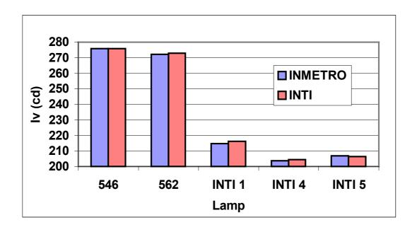
Figure 1: Results of luminous intensity comparison between INMETRO and INTI
