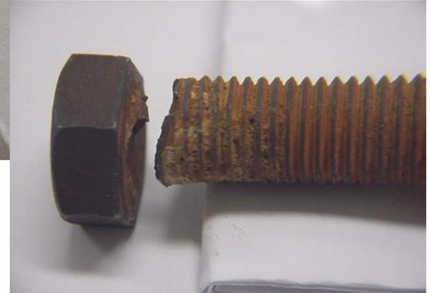
(HSCC - HYDROGEN STRESS CORROSION CRACKING)
